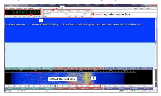
When logging a QSO, Fldigi calculates the true frequency (#3 in picture) by adding the offset (#2 in picture) to the transceiver dial frequency (#1 in picture). Without CAT, this frequency must be manually changed to the correct value by left or right clicking of the mouse. Each digit must be changed individually – a real pain!
