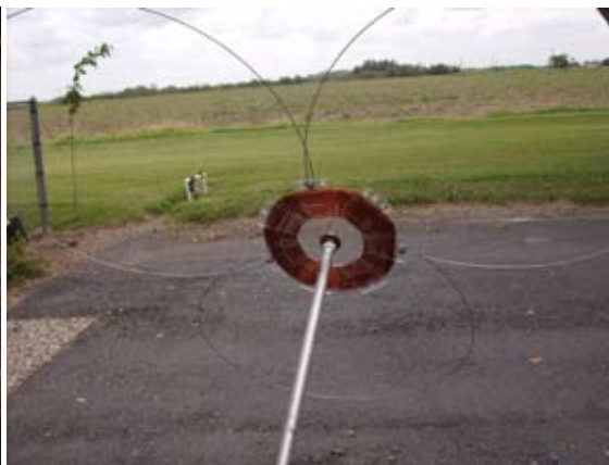
First for 160-It resonated at 960 kHz
